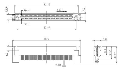
Figure 4.22 SCA2 type SCSI connector
